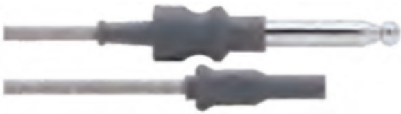
Silicone Monopolar Endoscopic Cable 10" (3.0m) SB-1503 Instrument Connector: 4.0mm Female Plug Generator Connector: Standard Bovie 8.0mm Plug Compatibility: Valleylab, Conmed, Bovie
